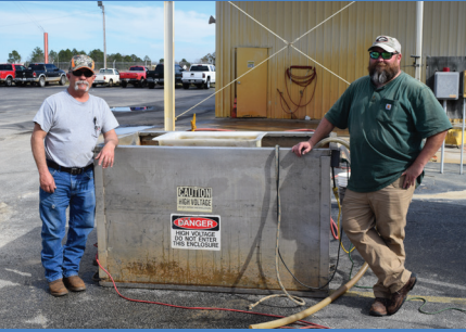
(Left to right) Technicians Chuck Reynolds and Billy Pump pose for a photo beside a water tank they use to test bucket liners. A liner is submerged in the tank and high voltage is applied to the water inside of the bucket liner for several minutes while water in the tank surrounding the liner is tested for voltage. If any voltage is recorded, the liner fails its test.
