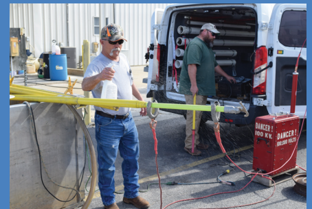
Chuck Reynolds sprays a solution on an extendable fiberglass pole while the high voltage testing board applies voltage to test the pole's electrical insulation value.
